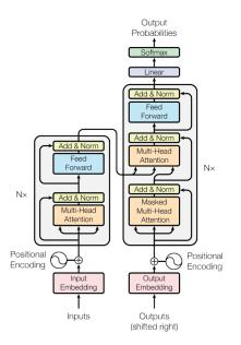
Fig. 1. The transformer - on the left side, the encoder, and on the right side, the decoder [8]
