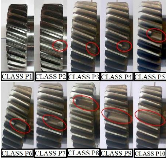
Fig. 4. All ten classes of gear tooth breakage [14].
