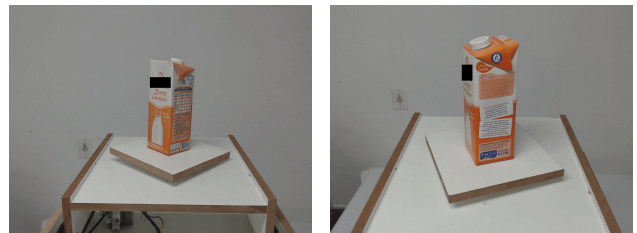
(a) Camera base original position (b) Camera base displacement 2 cm
