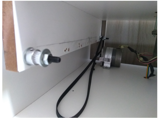
Fig. 9. Steeper motor fixed in the structure.
