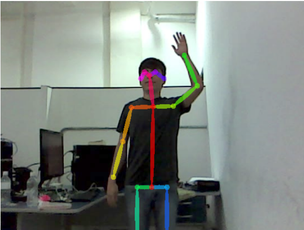
Fig. 5: A scene of the video processed by OpenPose used in the experiment.
