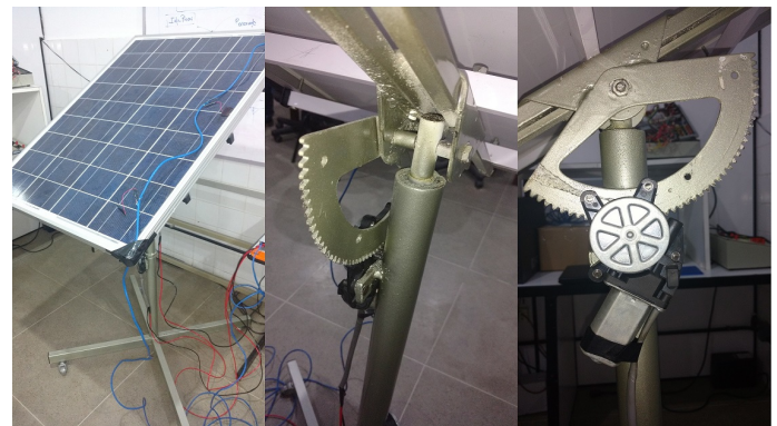
Fig. 8. Solar Panel and movement Gear of 3D table
