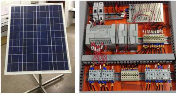
Fig. 6. Solar Position Tracking System
