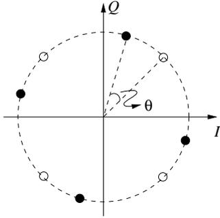
Figure 2: QPSK constellation: without rotation ( $\circ$ ); with rotation ( $\bullet$ ).
