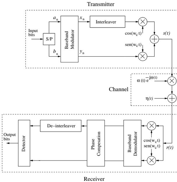
Figure 3: Block diagram of the communication system.
