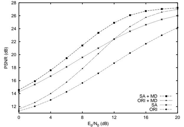
Figure 5: PSNR of the reconstructed Lena images as a function of the channel signal-to-noise ratio ( $E_b/N_0$ ), considering a codebook with 256 codevectors.
