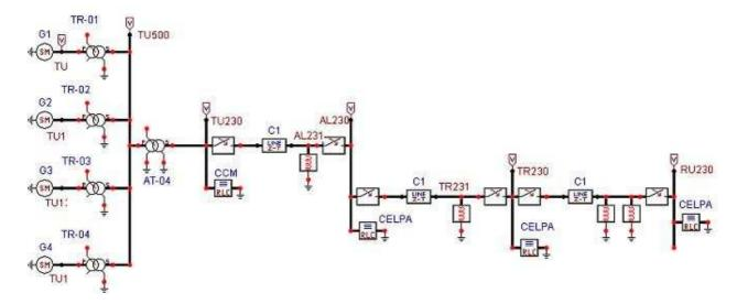
Fig. 4. The Eletronorte's Tramoeste system, which was used as the master ATP file for the illustrative example.
