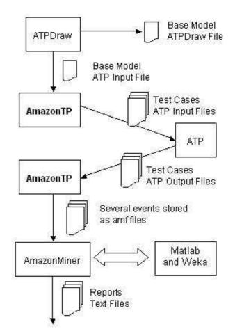
Fig. 2. The files generated along the whole process.
