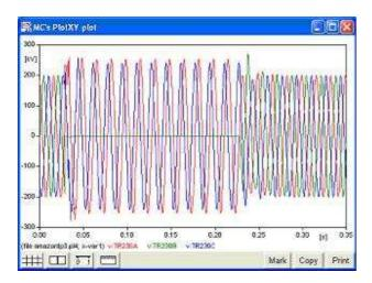
Fig. 5. Zoom of waveforms at the moment of a BT-fault generated by AmazonTP.
