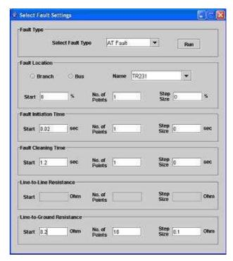
Fig. 3. Dialog window of the user-defined fault generation agent. The user can select the type of fault, its location and other parameters
