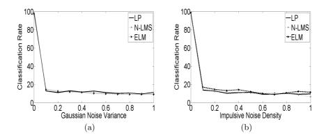
**Fig. 2.** Performances of linear and nonlinear neural classifiers to test images (SUSSEX) corrupted by (a) gaussian and (b) impulsive noise.
