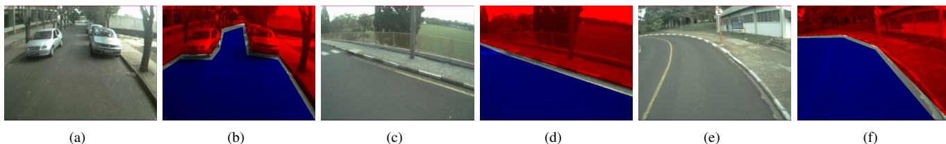
Figura 4: Samples of manual classification to generate the learning database. Images (a)(c)(e) are original images, images (b)(d)(f) are images manually labeled. The pixels painted of red represent pixels that classifier must returns non-road class. Pixels painted of blue represents pixels that classifier must return road class.
