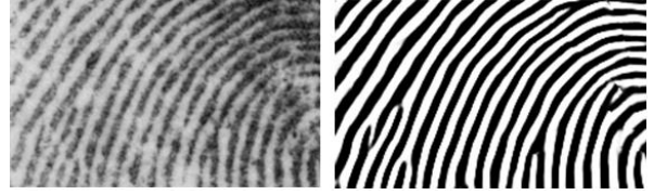
Fig. 11 – A fingerprint image and the respective image obtained through the Gabor filtering simulation using the proposed approach
