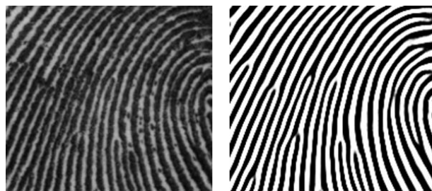
Fig. 7 – The left picture is a fingerprint fragment. The picture on the right is the result of the application of the method proposed in Hong, Wan and Jain [1]
