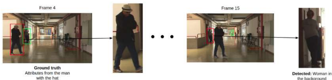
Figure 6: Detection using the SSD network. The video has the label for the attributes of the man with the hat (this is the ground truth). In Frame 4, the model detects two individuals, and the selected individual is ground truth. However, the model does not detect the ground truth individual that the video was labelled for in some frames (e.g. Frame 15).
