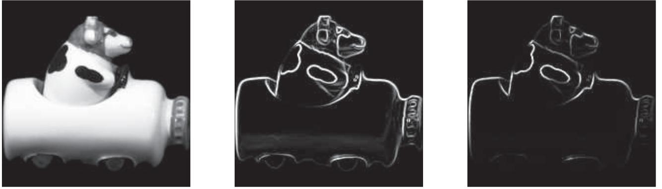
Figure 8: Input image  $I$  (left) and output images of normalized gradient  $|\nabla(I)|$  (center) and Sobel filter  $|S_{3 \times 3}(I)|$  (right).
