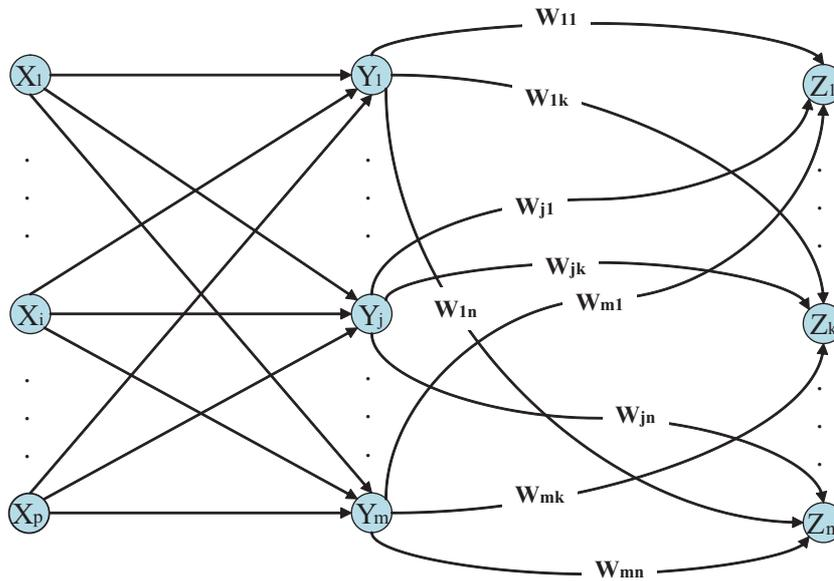
Figure 1: Backpropagation MLP architecture with one hidden layer.
