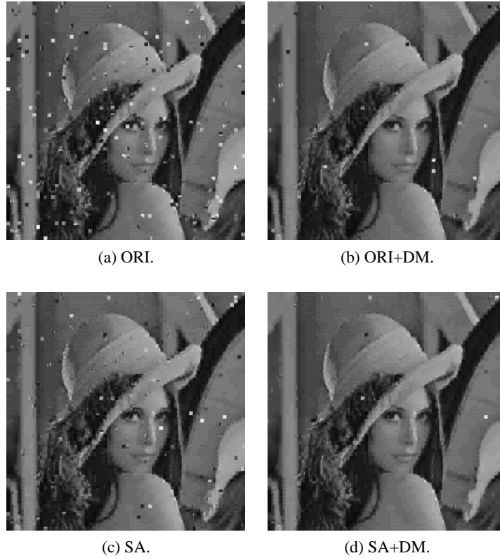
Figure 10: Reconstructed Lena image (VQ with 0.5 bpp) after transmission through a Rayleigh fading channel with E_b/N_0 = 16 dB.
