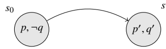
Figure 8: Representation of the states before and after a transition in a Kripke structure.
