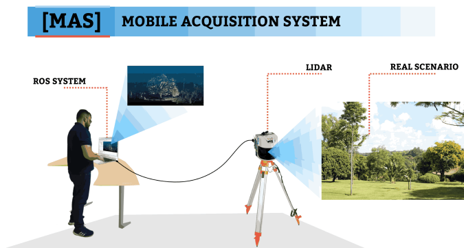
Figure 3: Mobile Acquisition System (MAS) Structure.
