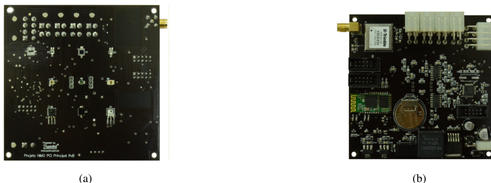
Figure 3: A picture of the implemented electronic board: (a) Top face: light sensors; (b) Bottom layer: main modules and analog conditioning circuits (extracted from [4]).
