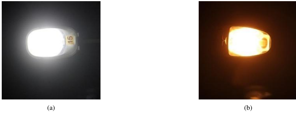
Figure 5: Photos of two different 150W street light bulbs: MH (a) and HPS (b)
